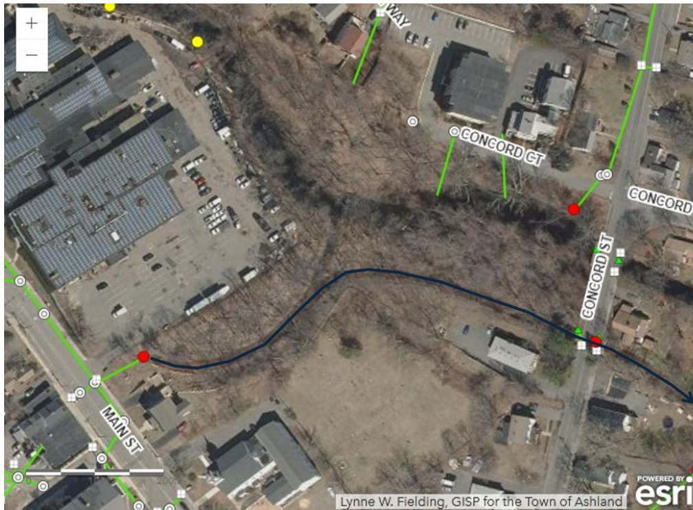
Figure 7: Ashland stormwater system map showing on the left side of the image the municipal outfall (red dot) from Main St. feeding the side stream (blue line) that was measured with high detergent levels. The Sudbury River is just north of the side stream.
