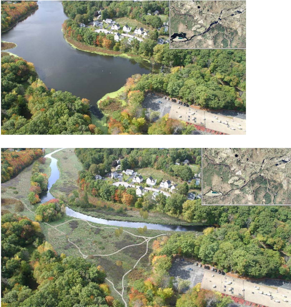
Figure 8. Ben Smith Impoundment Before and After Hypothetical Dam Removal
