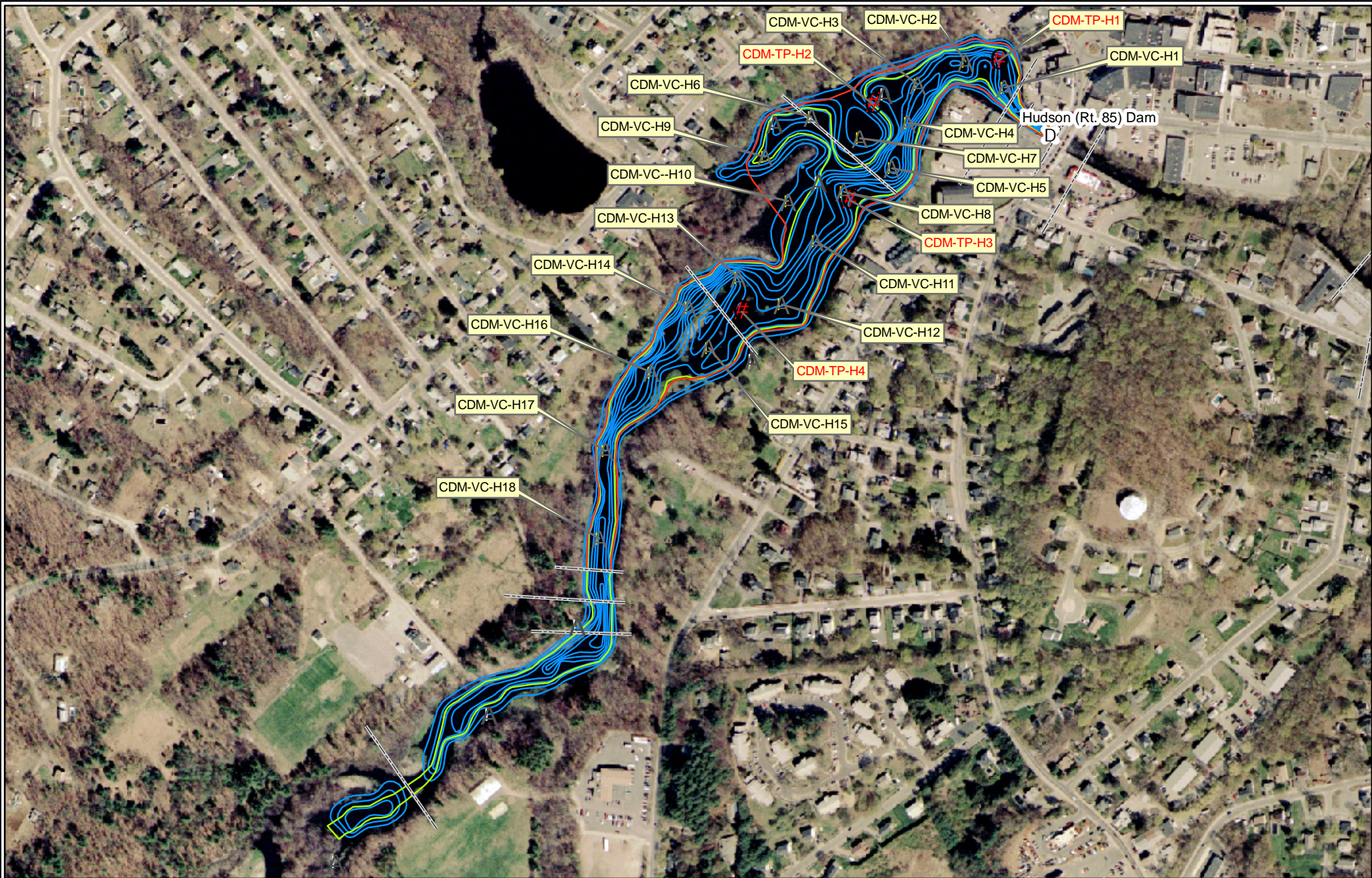
Figure 3-3: Proposed Subsurface Exploration Plan Hudson Impoundment
