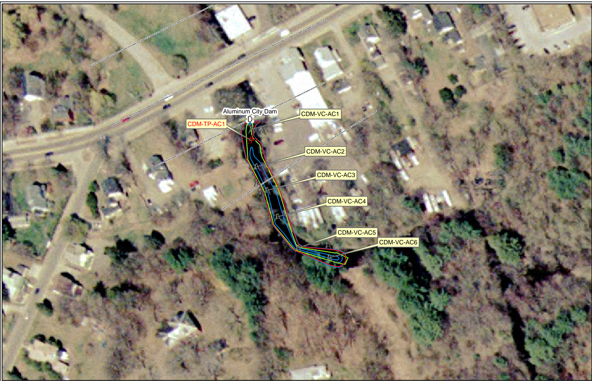
Figure 3-1: Proposed Subsurface Exploration Plan Aluminum City Impoundment
