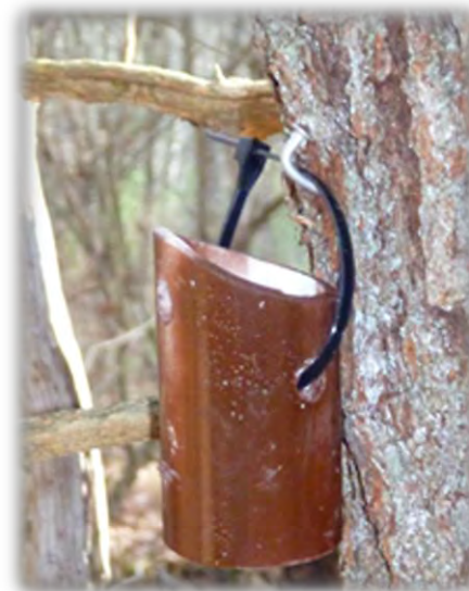
Figure 9: Air temp. logger installation
